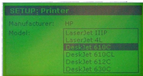
Using the keys "Cursor Up" and "Cursor Down" select the manufacturer of the printer you are using with the instrument. Confirm your selection with the "Enter" key.
