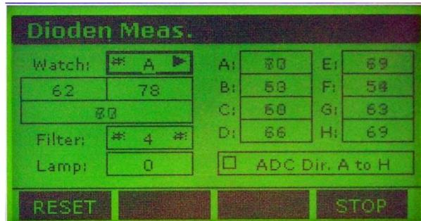
Select the lowest wavelength filter from the ‘Filter:’ selection window as you will be using the lamp at near maximum brightness. If you cannot use a filter then manually turn the filter wheel to block the light reaching the fibre optic loom.
