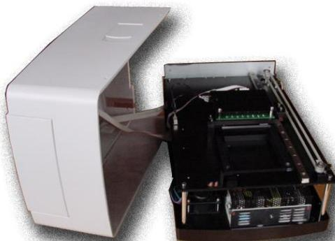
The cover is now connected to the instrument by the display and keyboard cables. To completely remove the cover, disconnect the two ribbon cables from the instrument.
