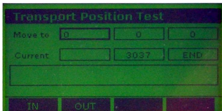
This menu allows you to define specific positions, to move the plate carrier and to manually step the transport in and out. Use the keys “**Cursor Up**” and “**Cursor Down**” to select the entry fields for “Move to”. Enter values (between 0 and 3037) using the numerical keys. After the requested position has been entered, you must confirm the value by pressing “**Cursor Up**” and then “**Cursor Down**” and then “**Enter**”
