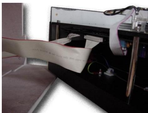
To re-assemble the cover, follow the above description in reverse order. Do not tighten screws until they have all been located in the corresponding threaded holes.
