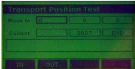
This menu allows to define specific positions to move the plate carrier to, to manually step the transport in and out.
