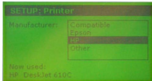
Using the keys "Cursor up" and "Cursor Down" select the manufacturer of the printer you are using with the instrument. Confirm your selection with the "Enter" key.
