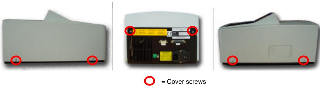
**1. DANGER: Switch off the instrument and disconnect the power cable.**
