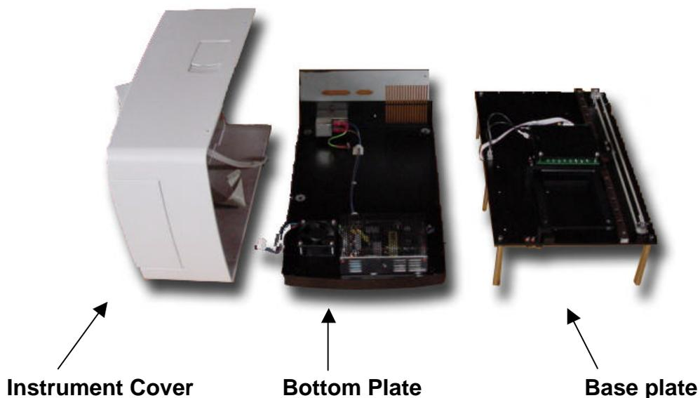
The **Instrument Cover** holds the keyboard and the display and contains the front lid (for light protection of optical system during plate reading) and the filter compartment lid (for easy access to the filter wheel).
