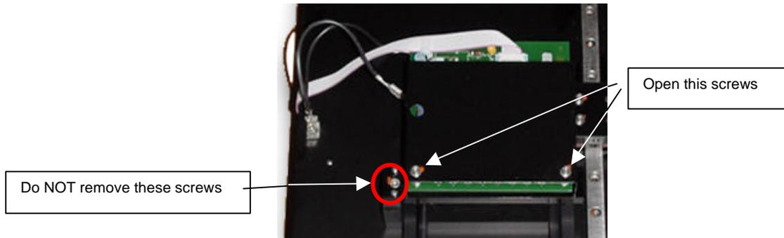
Open the hex screws as marked above and lift board from the instrument. Mount the new board in reverse order.
