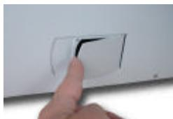
The filters are held in place on the filter wheel by spring wires and can easily be replaced without using tools.
