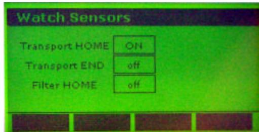
This screen shows the actual status of all three sensors of the instrument. The instrument has three sensors: Transport Home, Transport End and Filter wheel.
