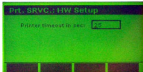
Use the numerical keys to enter the required printer timeout.
