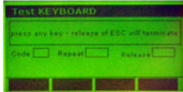
Pressing any key will insert the code of the respective key into the field “Code”. As long as the key is being kept pressed, the field “Repeat” will keep increasing. As soon as the pressed key is being released, there will be displayed a “YES” in the field “Release”.
