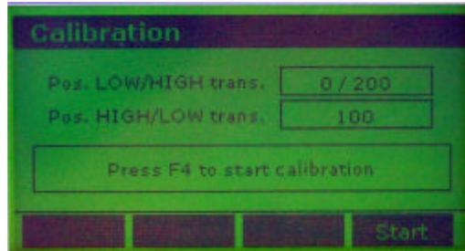
Pressing “F4” will calibrate the Filter wheel home position sensor.
