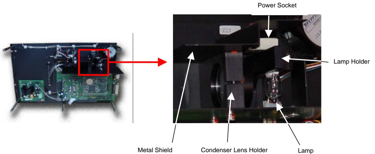
1. Remove the metal shield (see graph above) by removing the two screws that are holding it onto the condenser lens holder
