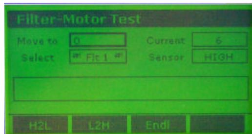
This menu allows to define specific positions to move the Filter wheel to, and to check the Filter wheel sensor.
