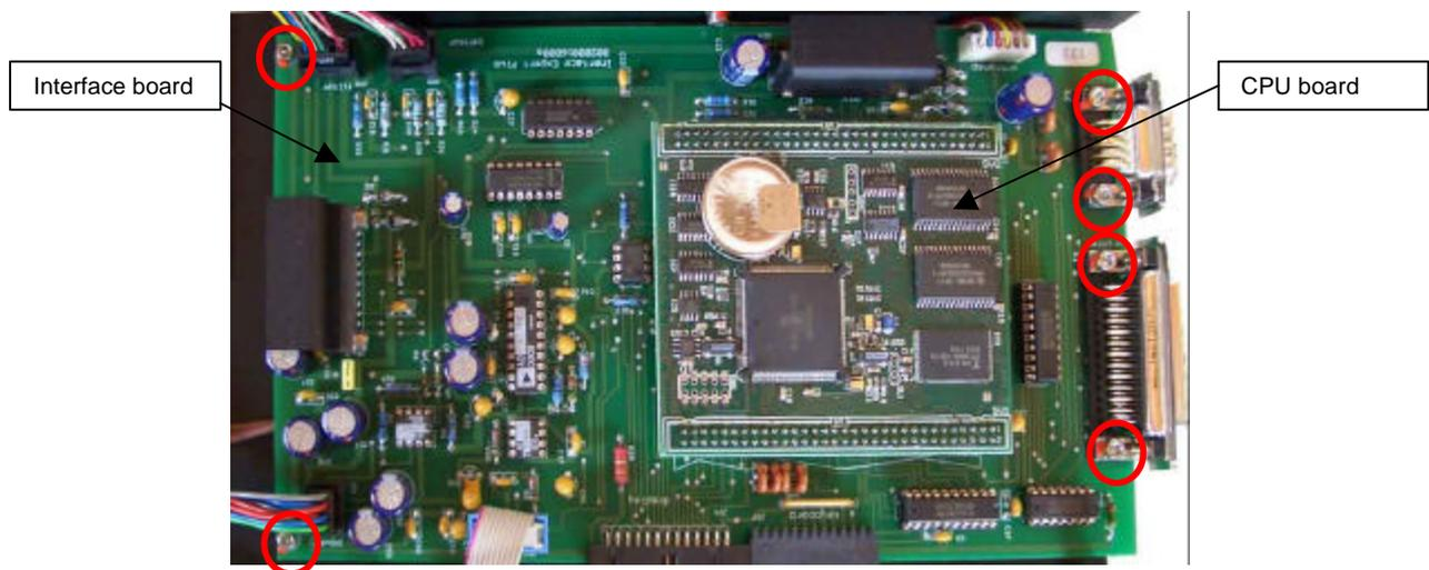
1. Carefully lift the CPU board from the connectors that hold it onto the Interface board.
