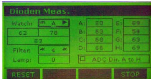
This menu allows to check each of the eight optical channels, with each of the available wavelengths, at selectable lamp intensity.
