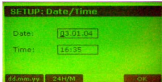
Press “ F1 “ to select between the available date formats (**dd.mm.yy** or **mm-dd-yy** or **yy/mm/dd**)
