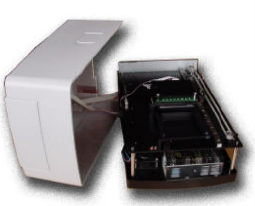
The cover is now only connected to the instrument by the Display- and Keyboard cables. To completely remove the cover, disconnect these two ribbon cables from the instrument:
