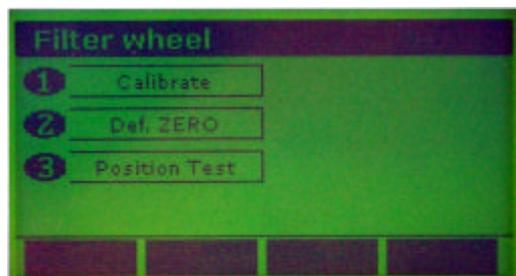
***ATTENTION:*** The Submenu “Define Zero” should never be opened, except after replacing the filter wheel sensor (see chapter [7.8](#)) !
