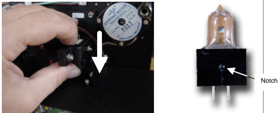
4. The lamp is held in the right position by a spring loaded ball, which is snapped into a notch on the lamp socket.
