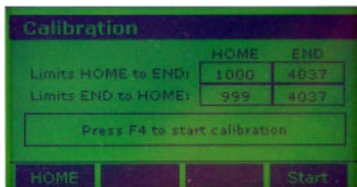
Pressing “ **F1** ” will move the transport to Home position (= out), pressing “ **F2** ” will move the transport to End position (= in).
