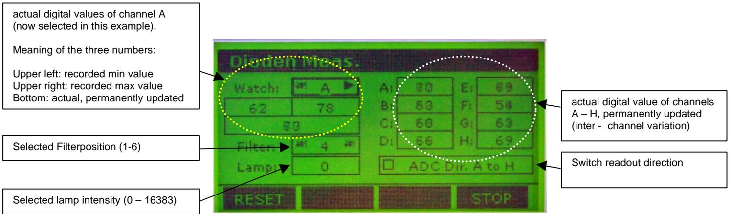
Use the keys **“Cursor up”** and **“Cursor down”** to select the entry fields **“Watch”**, **“Filter”**, **“Lamp”** and **“ADC Dir. A to H”**.
