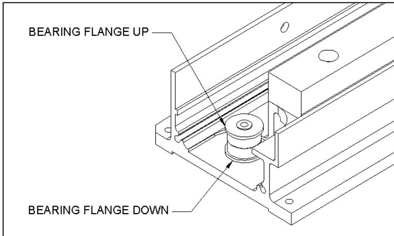
Figure 7-50 Replacing the Idler Pulley
