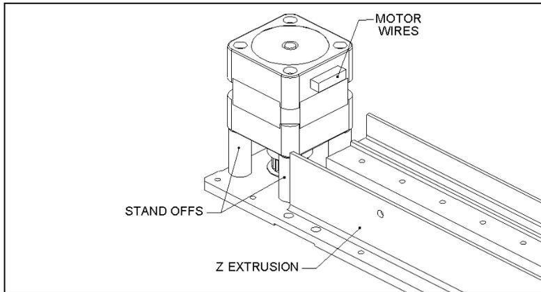
Figure 7-29 Replacing the Motor Assembly
