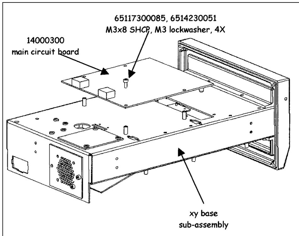
Figure 9-8 Mounting the Main Circuit Board
