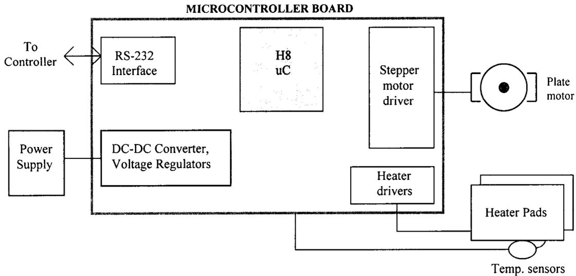
Figure 8-1 Circuit Block Diagram - Incubator Module
