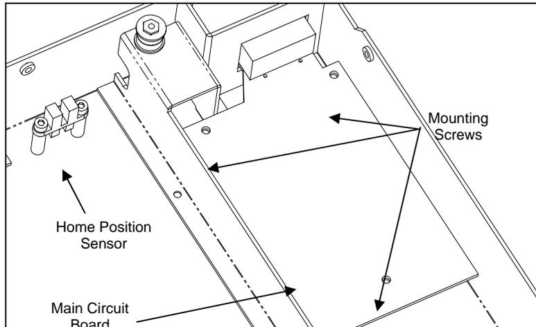
Figure 15-9 Ambient Drawer Main Assembly PCB
