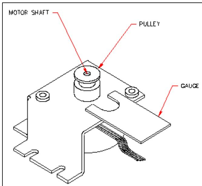
Figure 9-17 Drive Pulley Mechanism
