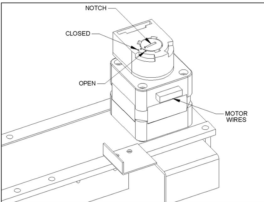
Figure 7-39 Positioning the Y-Axis Encoder
