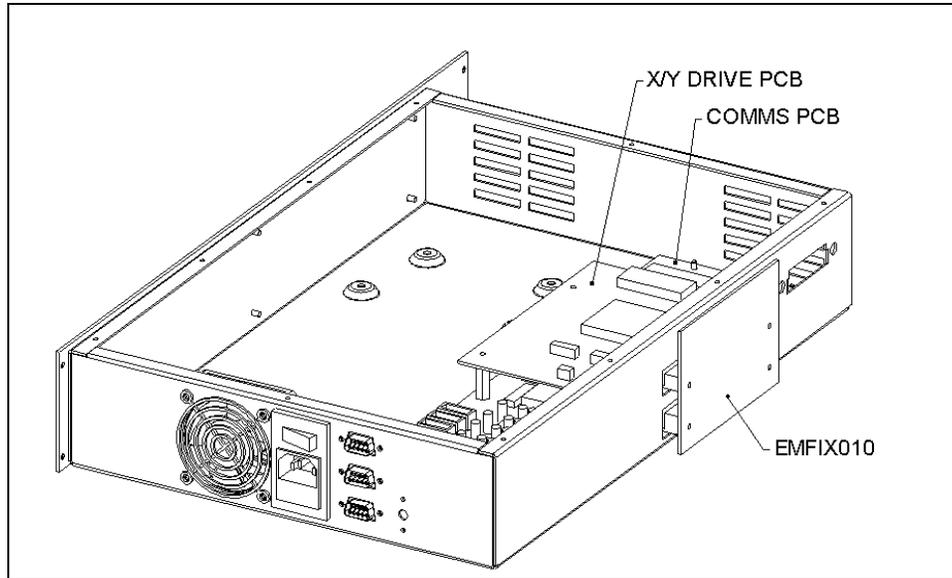
Figure 17-9 Aligning the Printed Circuit Boards
