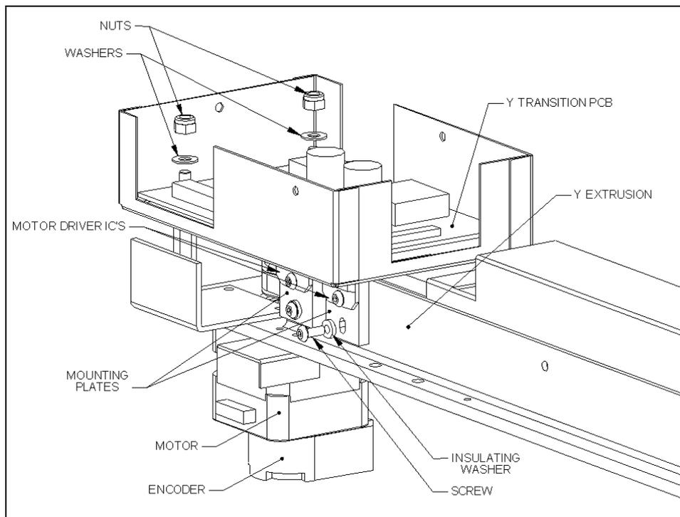
Figure 7-36 Y Transition Board Mounted in EMC Box
