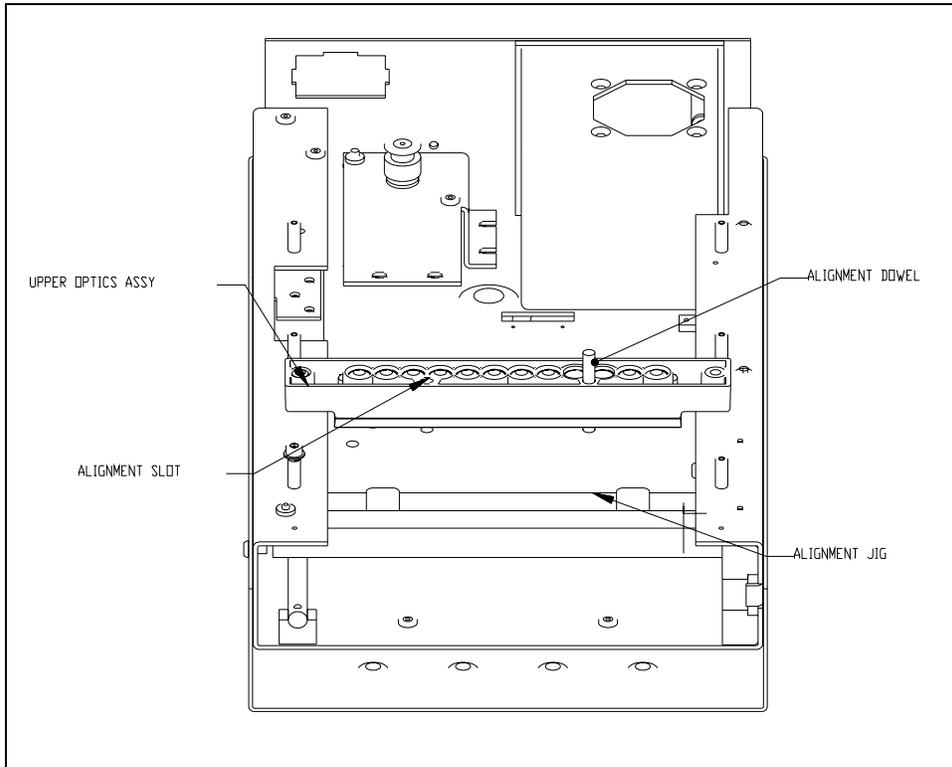
Figure 11-44 Alignment of Upper Optic Assembly
