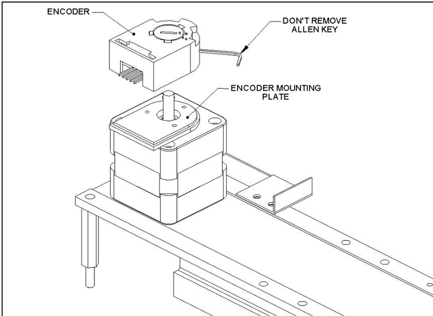
Figure 7-38 Mounting the Y-Encoder
