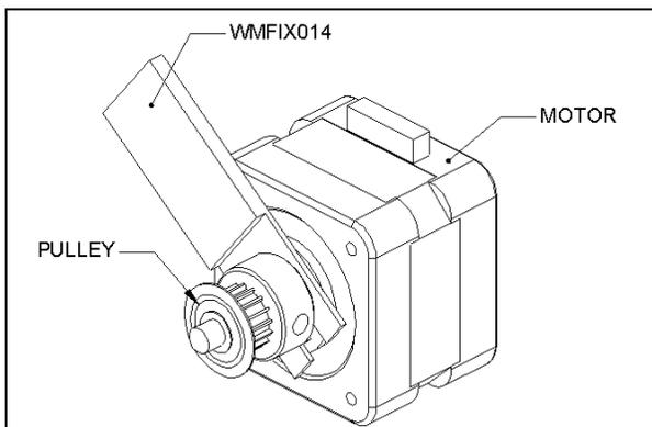
Figure 13-22 Positioning the Pulley on the Z-Drive Motor
