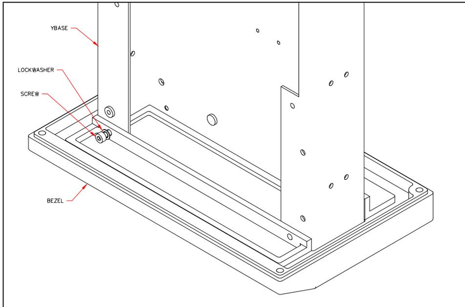
*Figure 9-3 Removing the Front Bezel*
