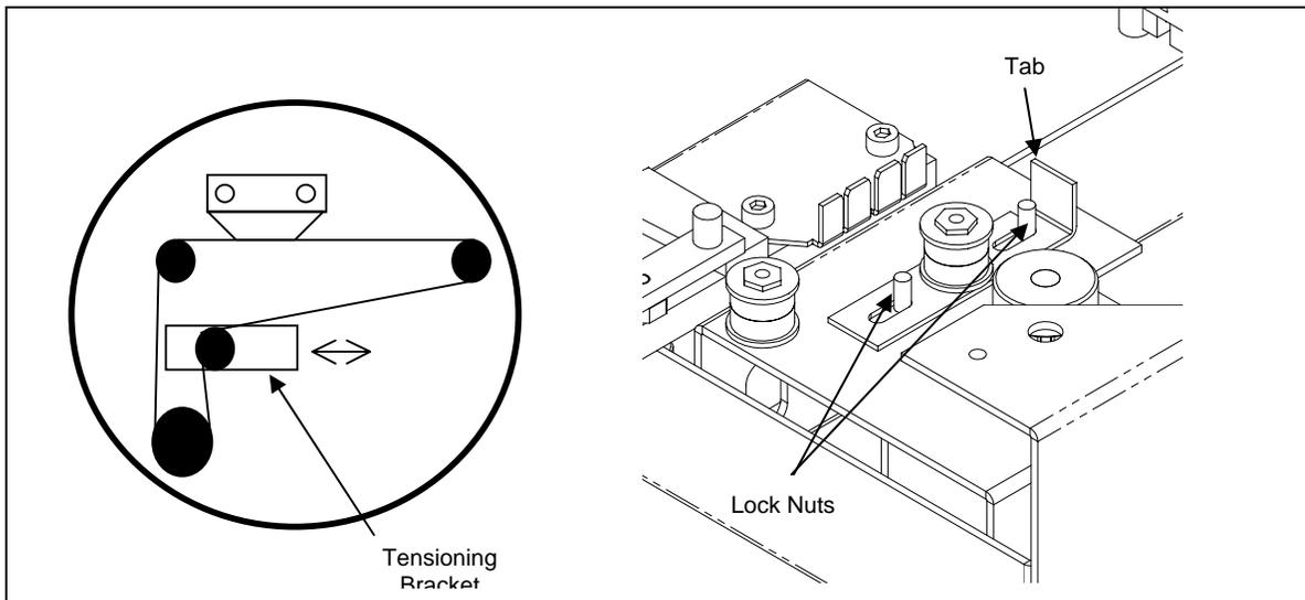
Figure 15-5 Tightening the Belt
