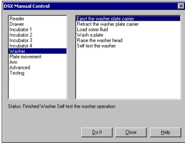
Figure 5-5 DSX Manual Control Dialog Box (Washer Selections)
