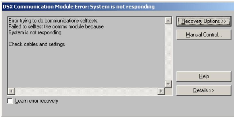
Figure 2-5 DSX Communication Module Error Dialog Box
