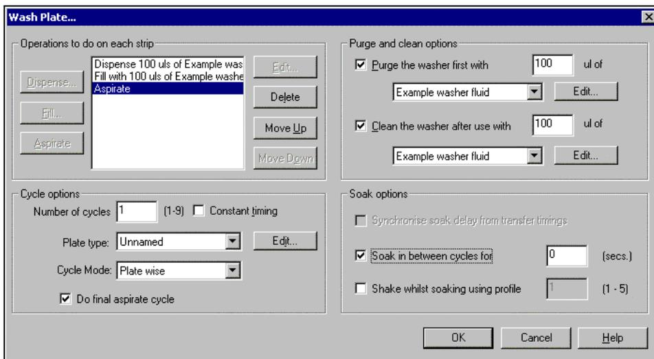
Figure 5-20 Typical Wash Plate Sequence
