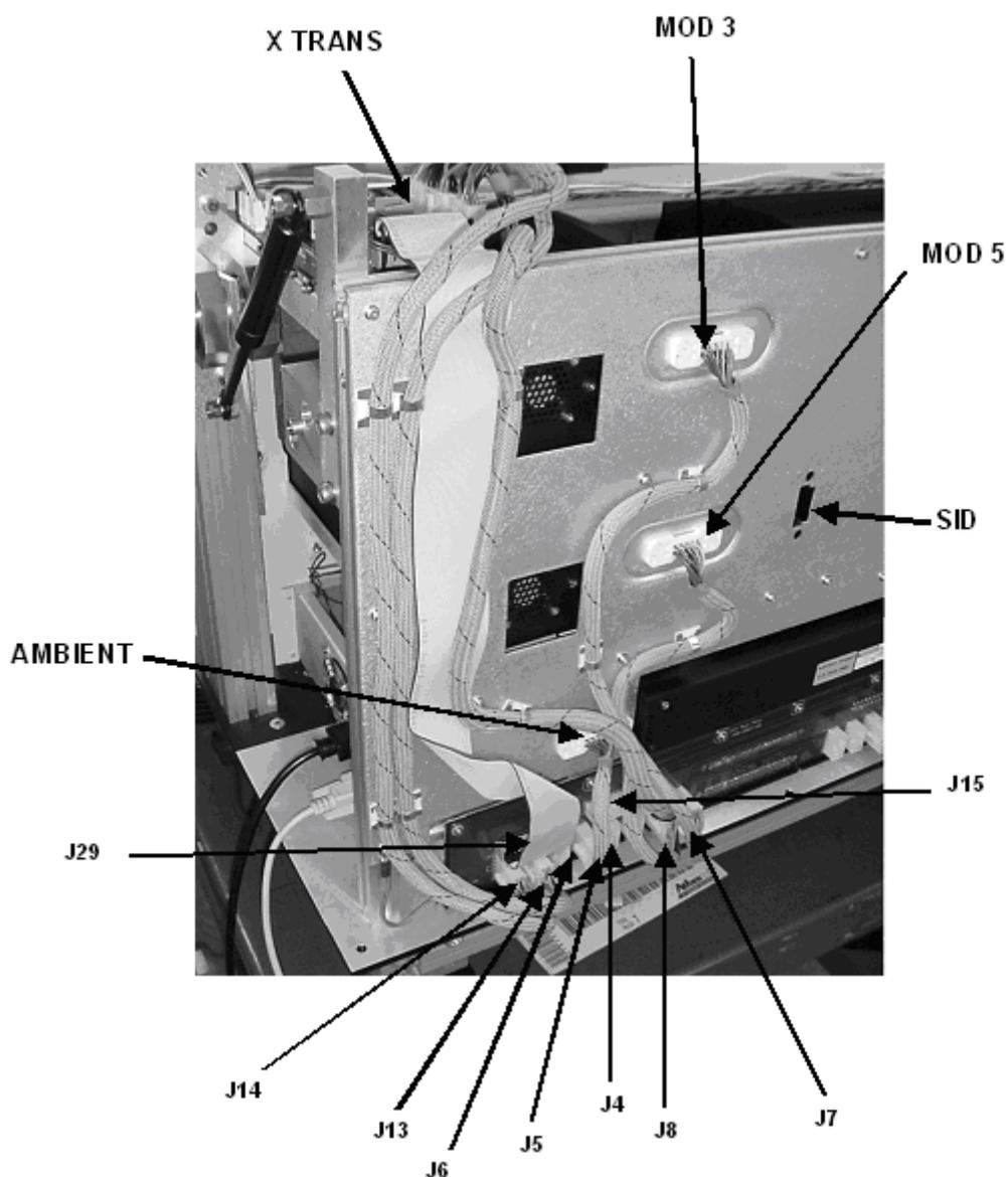
Figure 17-17 Back Panel Cabling - Panel 2
