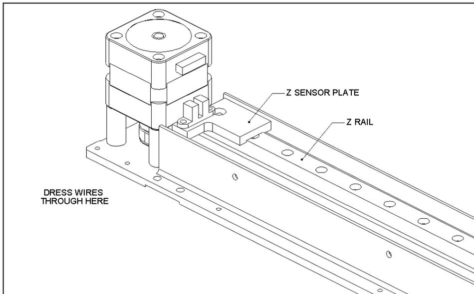
Figure 7-20 Z-Axis Sensor Plate
