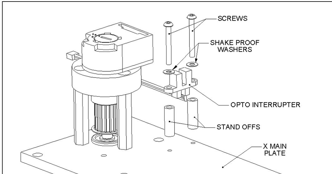
Figure 7-51 X Axis Optointerrupter
