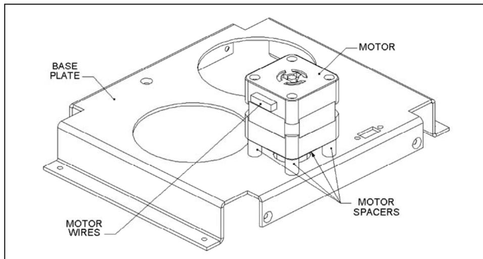
Figure 13-30 Y Motor Assembly.
