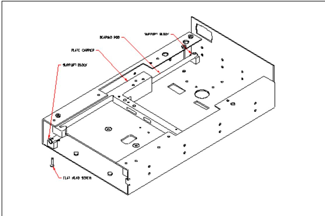
Figure 9-19 Mounting of the Plate Carrier Assembly
