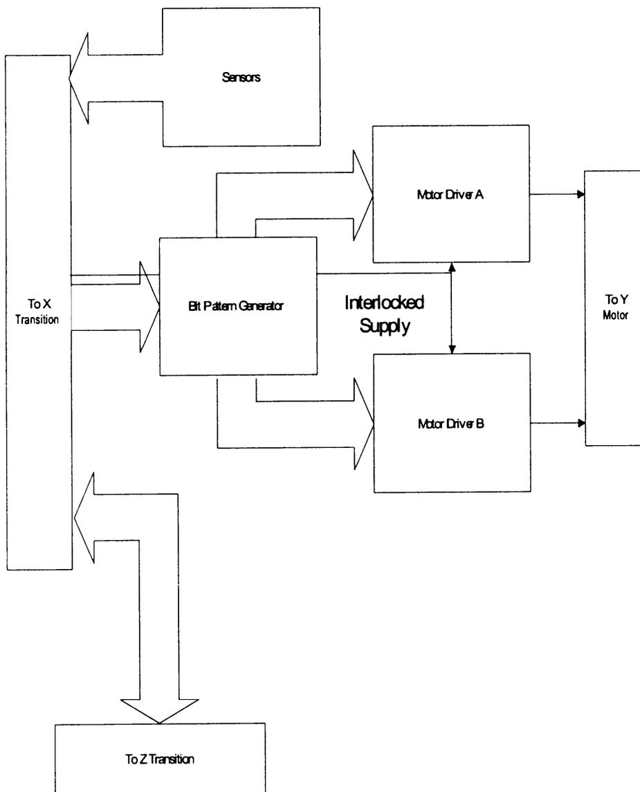
Figure 6-4 Y Motor Drive Transition
