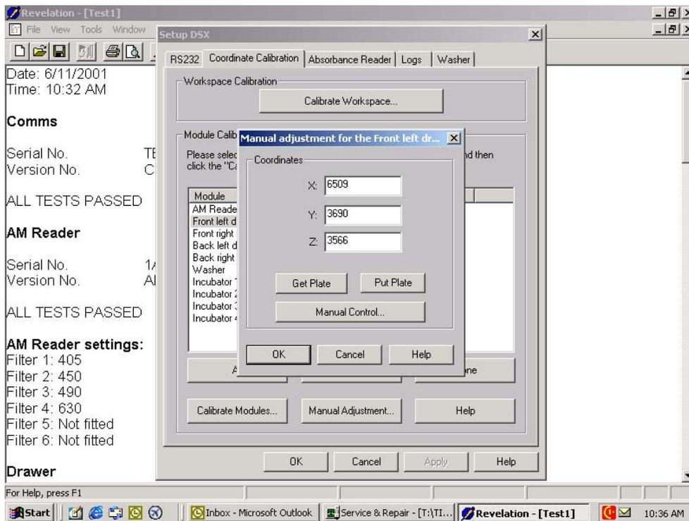
Figure 3-5 Front Left Drawer Manual Adjustment Dialog Box.
