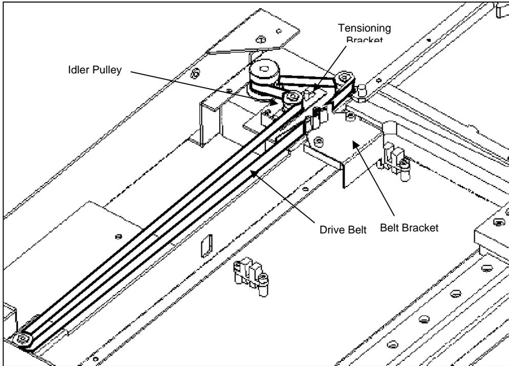
Figure 15-2 Timing Belt Bracket, Idler Pulley, and Tensioning Bracket
