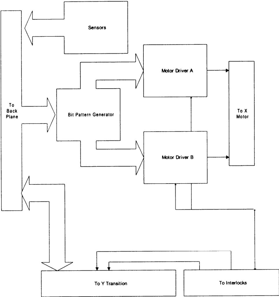
Figure 6-3 X Motor Drive Transition
