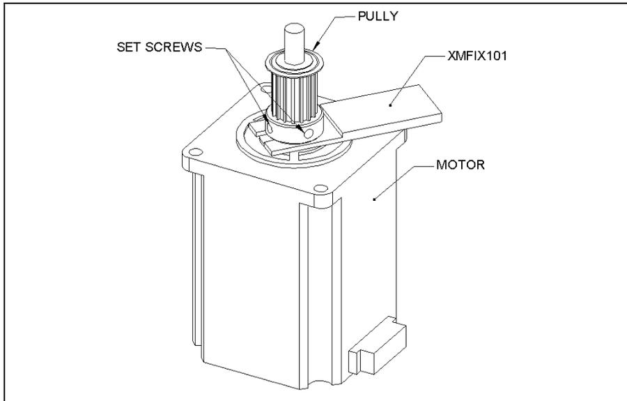
Figure 7-56 Affixing the Pulley to the X-Drive Motor
