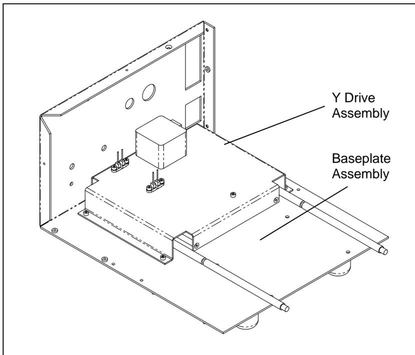
Figure 13-14 Installing the Wash Y-Drive Assembly
