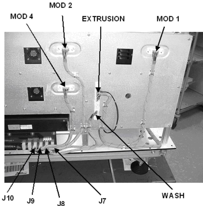
Figure 17-16 Back Panel Cabling - Panel 1
