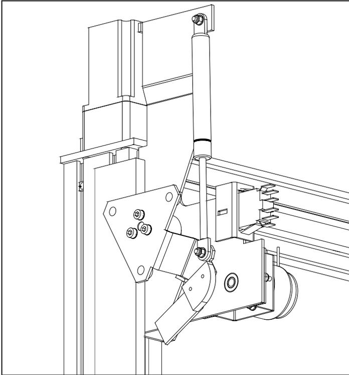
Figure 16-9 Mounting of the Gas Damping Spring
