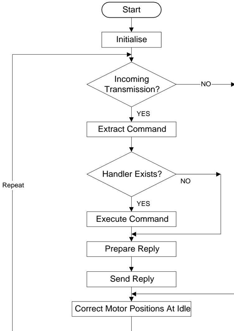
Figure 6-6 Top-Level Functional Design XY Program
