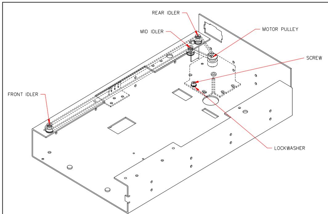
Figure 11-11 Plate Carrier Drive
