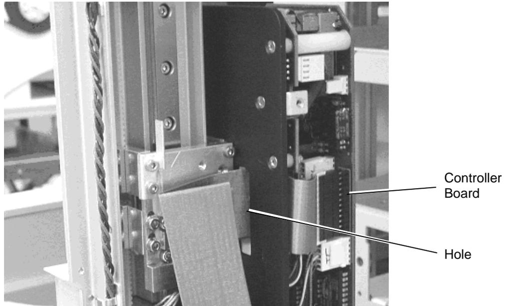
*Figure 7-2 Unplugging the Cable from the Controller Board*
