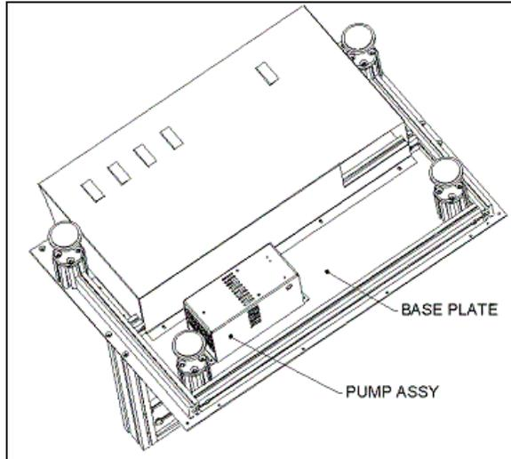
*Figure 13-5 Aspirate Pump Assembly*
