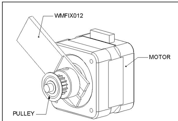
Figure 13-18 Positioning the Pulley on the X-Drive Motor
