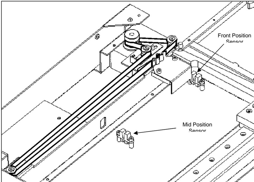
Figure 15-10 Location of Front and Mid Optical Position Sensors
