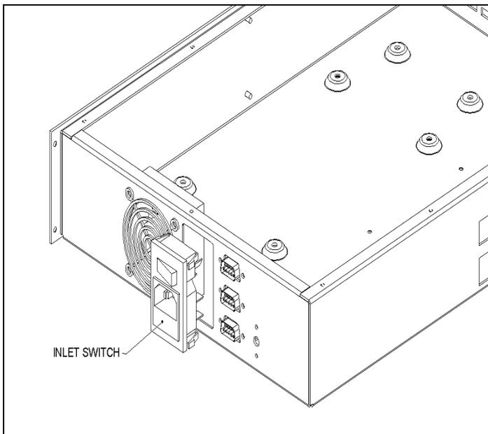
Figure 17-5 Inlet Switch Position
