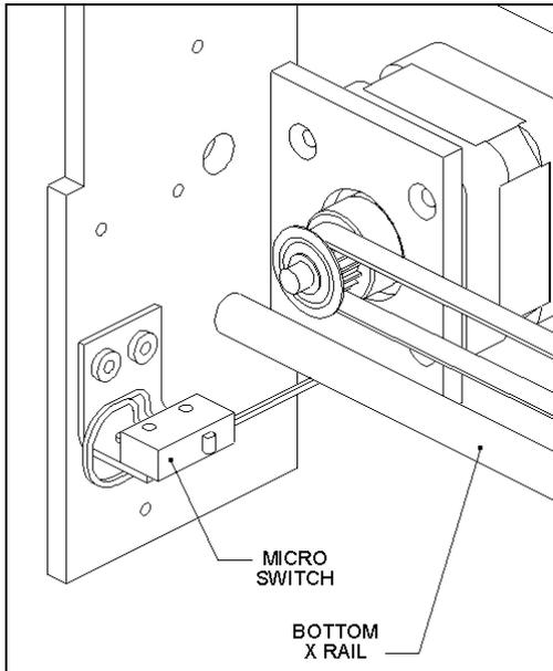
Figure 12-2 X-Motor Mounting Detail
