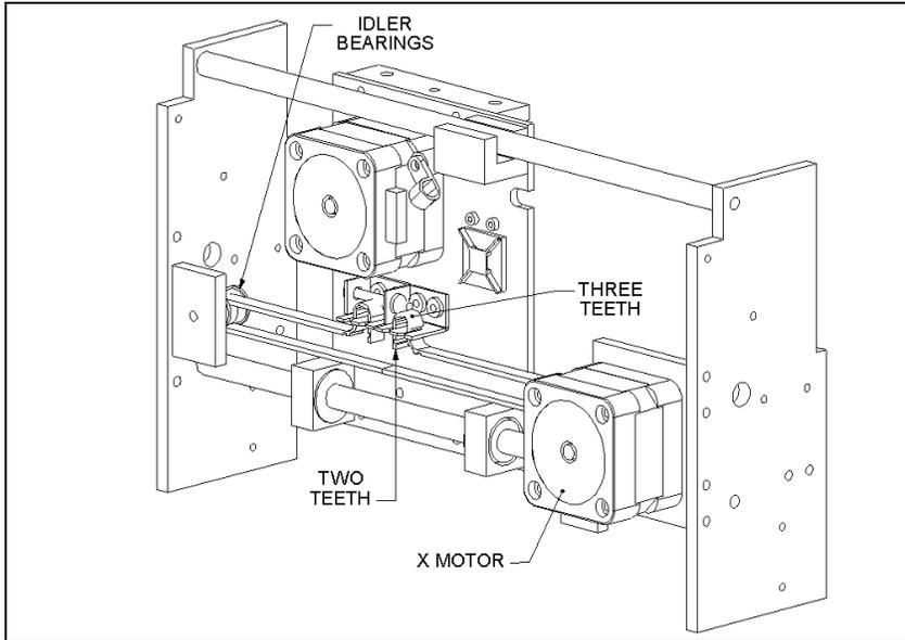
Figure 13-19 X-Drive Belt Installation
