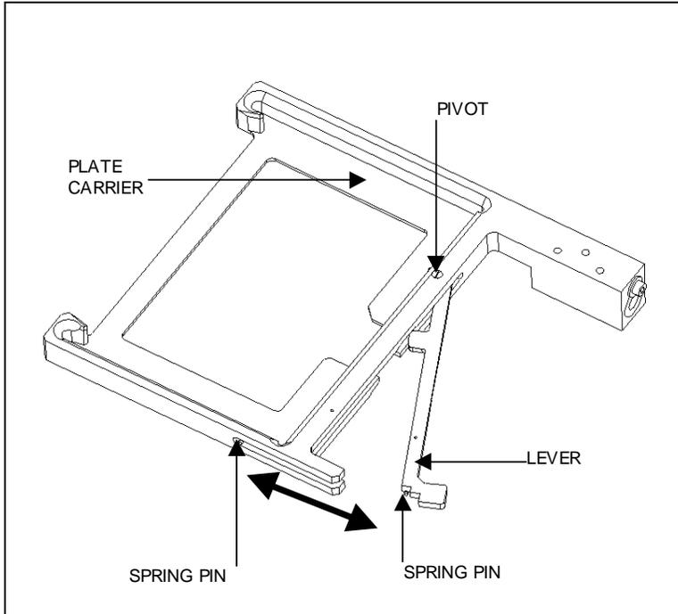
Figure 11-17 Locking Lever/Pivot and Spring
