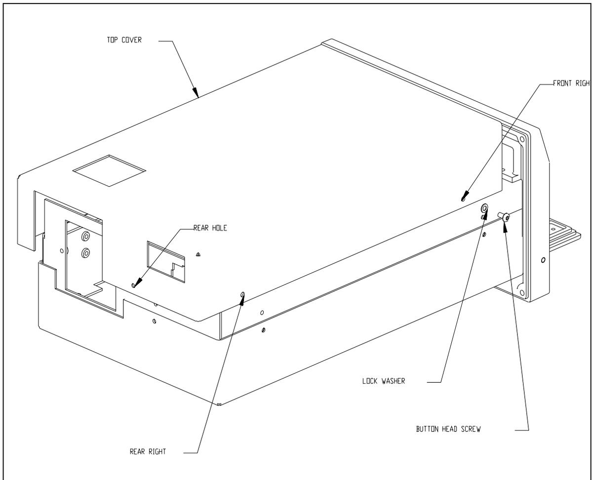
Figure 9-1 Removing the Top Cover
