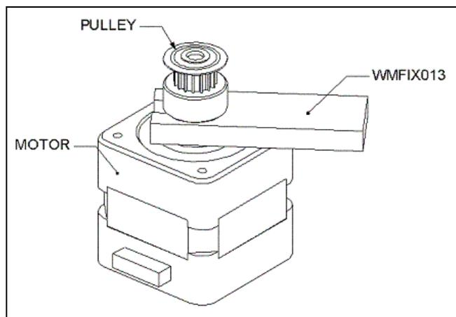
Figure 13-31: Attaching the Motor Pulley
