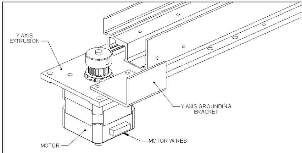
Figure 7-49 Mounting the Y Axis Motor
