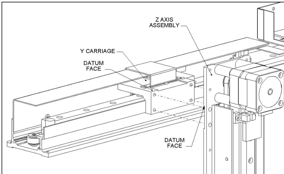
Figure 7-13 Mounting the Z-Drive Assembly
