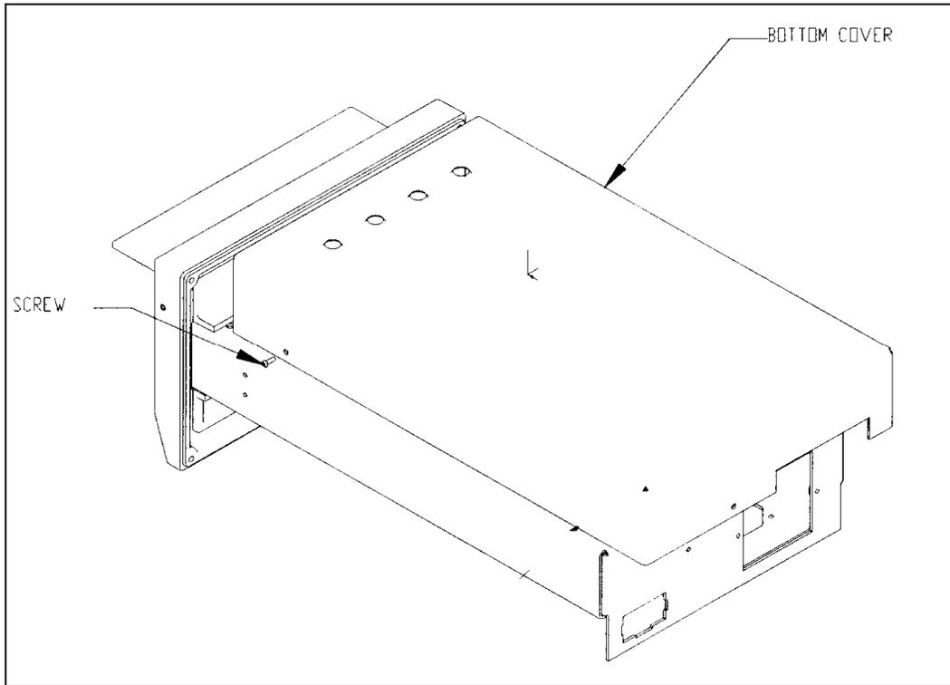
Figure 9-2 Removing the Bottom Cover
