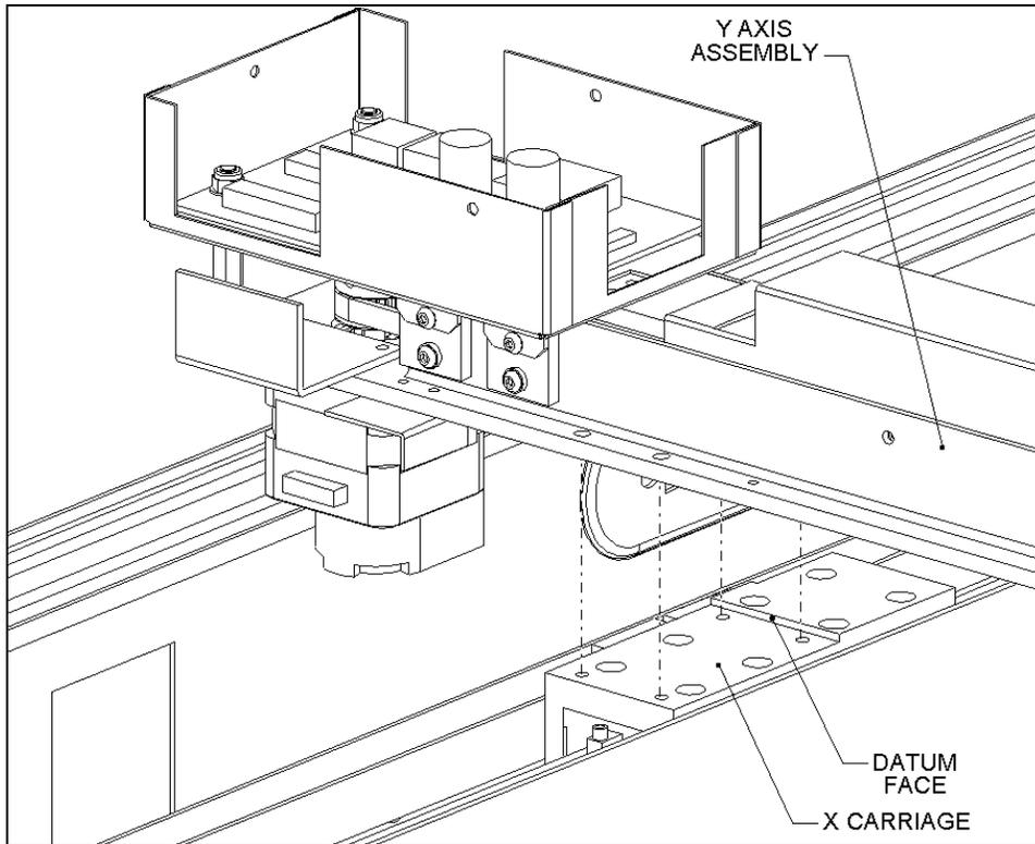
Figure 7-35 Mounting the Y-Drive Assembly on the X-Drive Assembly
