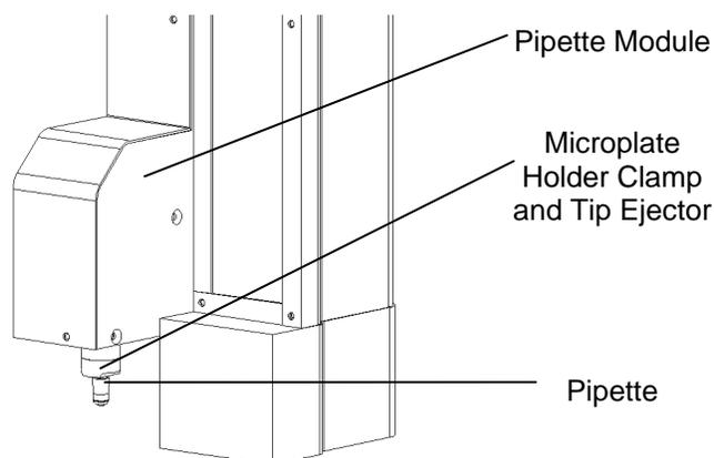
Figure 1-6 Pipette Module
