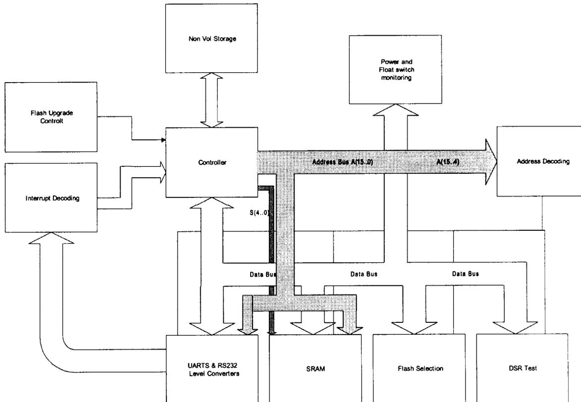
Figure 17-2 Circuit Block Diagram for the EPOD
