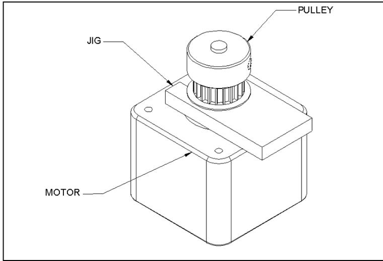
Figure 7-48 Replacing Motor Pulley
