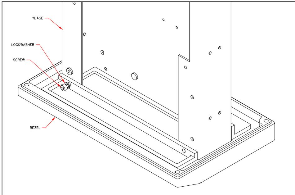
*Figure 11-5 Removing the Front Bezel*
