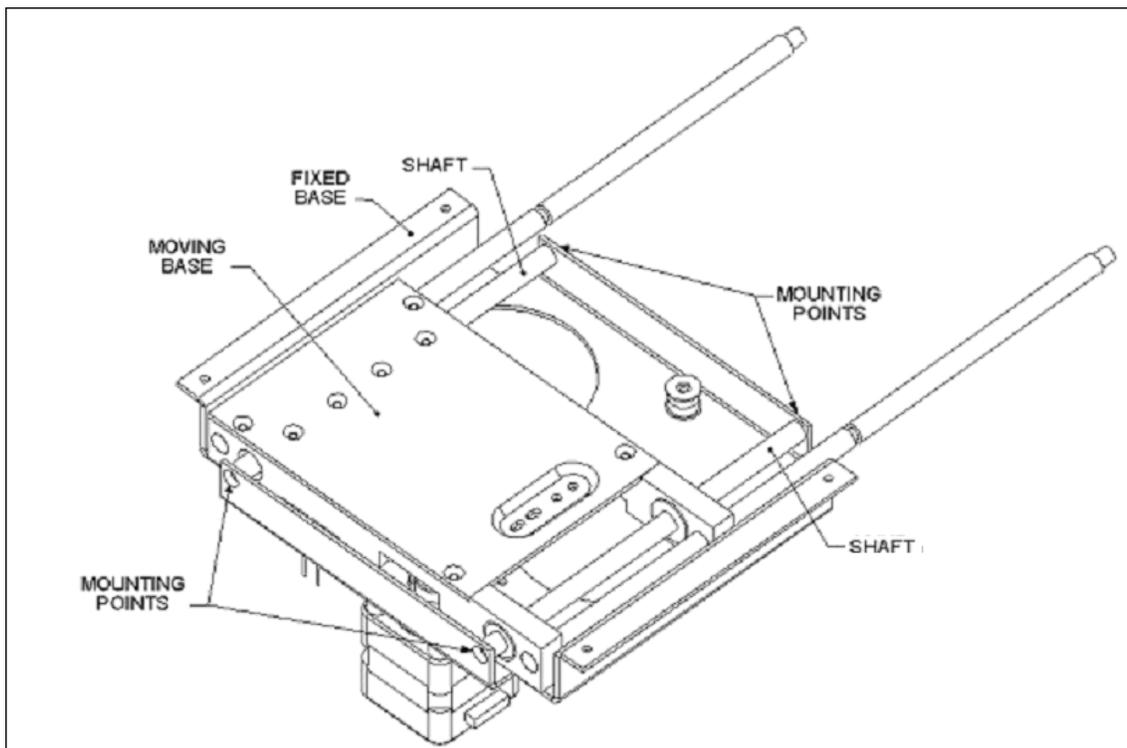
Figure 13-27 Mounting Moving Base Assembly Fixed Base Assembly
