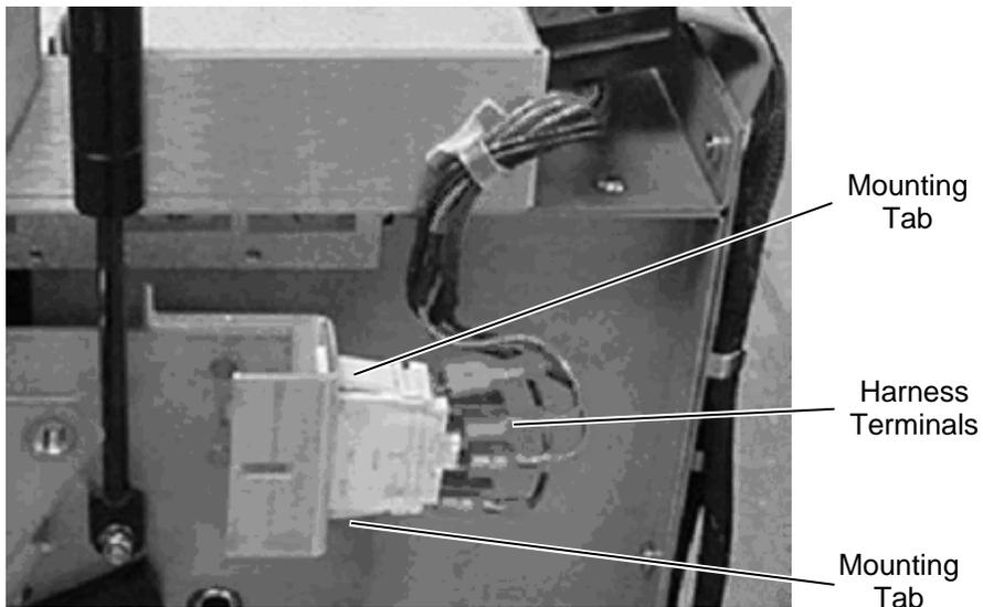
Nut *Figure 16-8 Interlock Switch*
