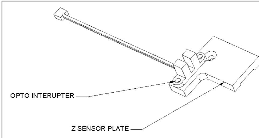
Figure 7-19 Z-Drive Optointerrupter Assembly
