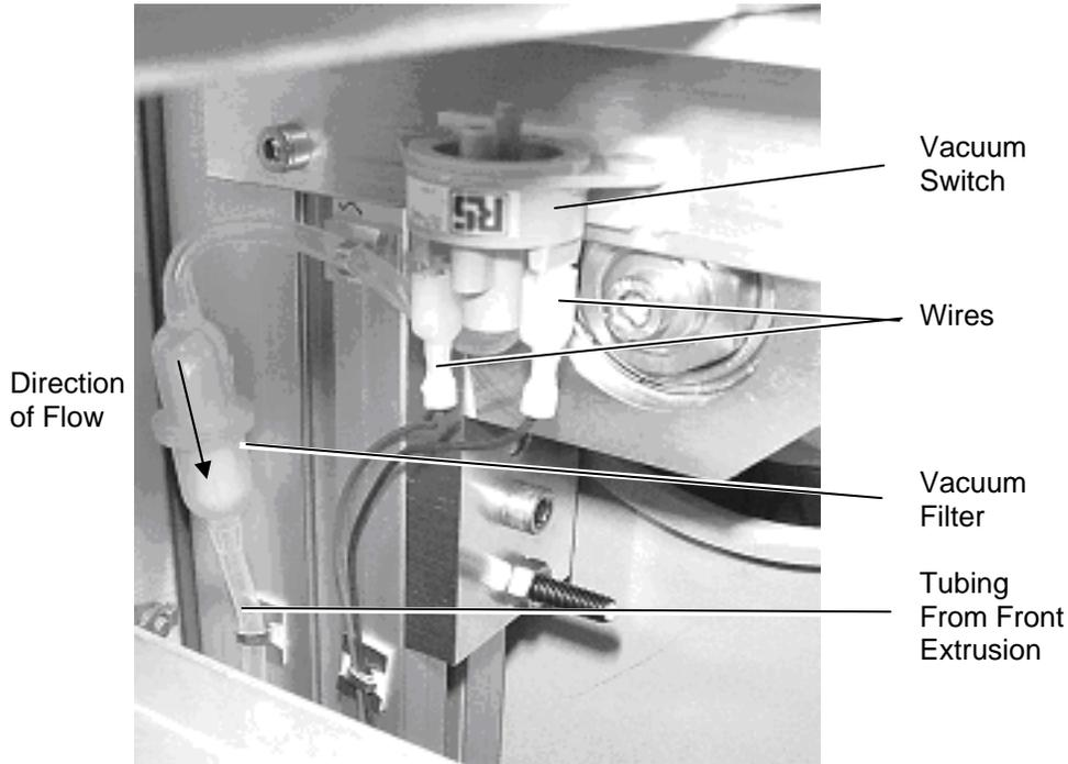
Figure 13-7 Vacuum Switch Parts
