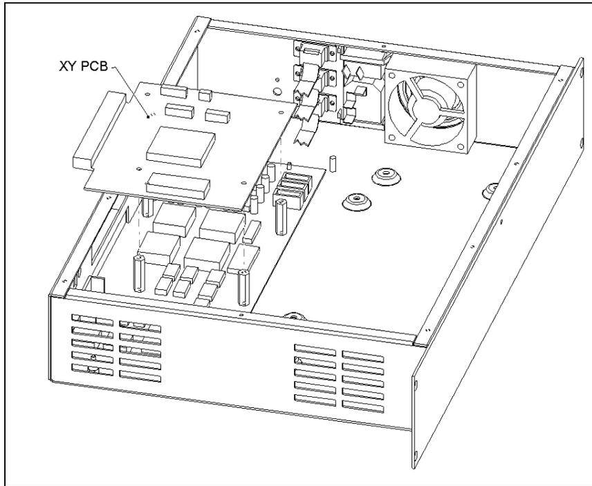
Figure 17-8 XY Printed Circuit Board
