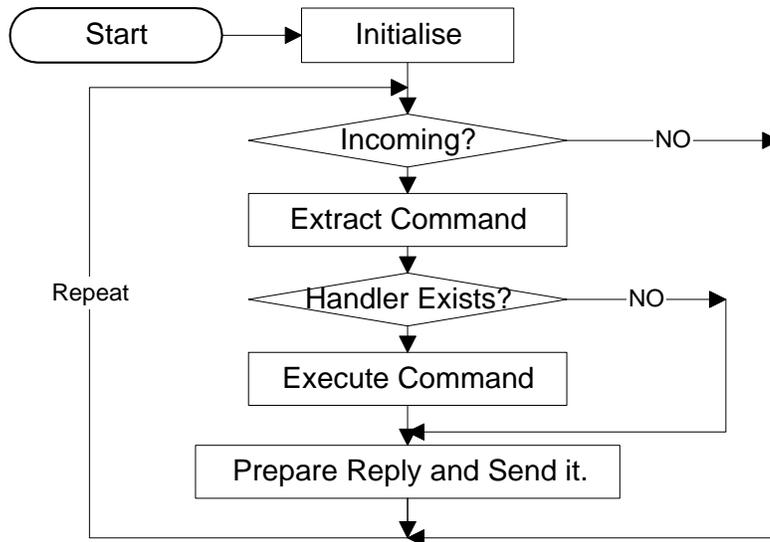
Figure 6-10 Top Level Z/Pipette Module Program
