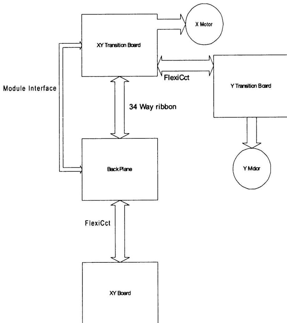
Figure 6-1 Circuit Board Diagram – Board Breakdown
