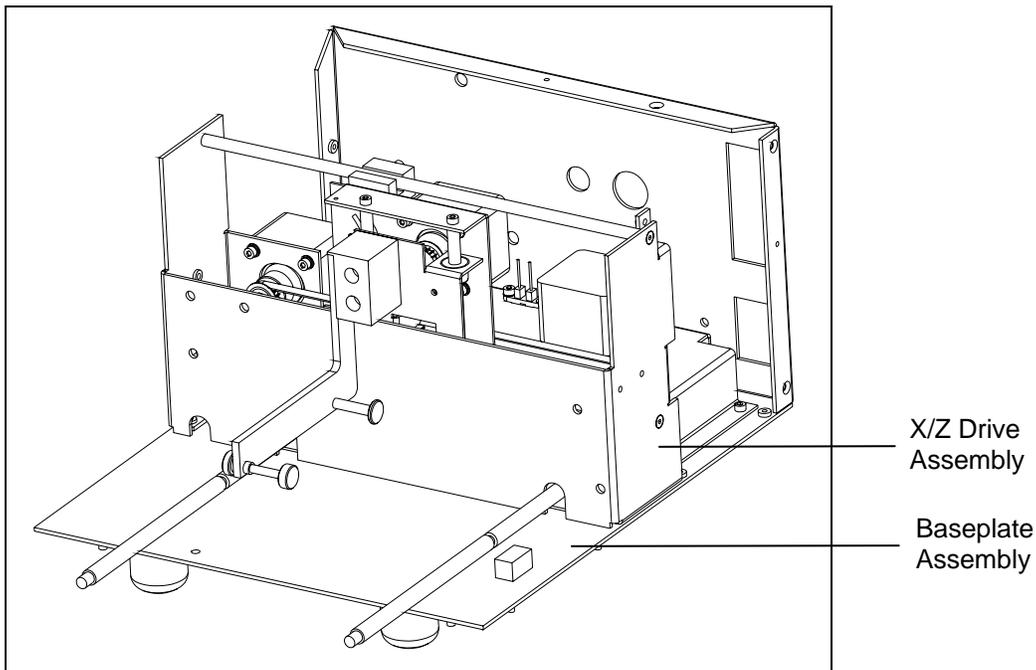
Figure 13-13 Mounting the Wash X-Z Subassembly
