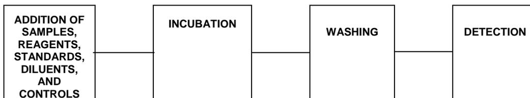
Figure 1-2 Operation Steps of the DSX™ Automated ELISA System
