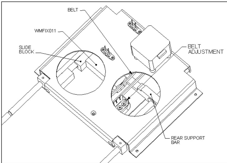
Figure 13-24 Y-Axis Assembly
