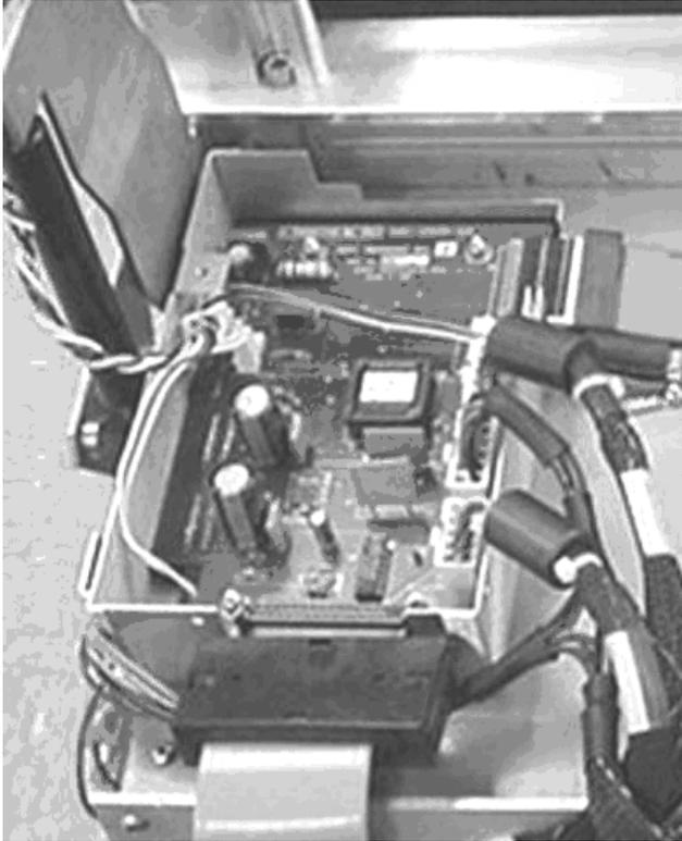
*Figure 7-61 Location of X-Transition Printed Circuit Board*
