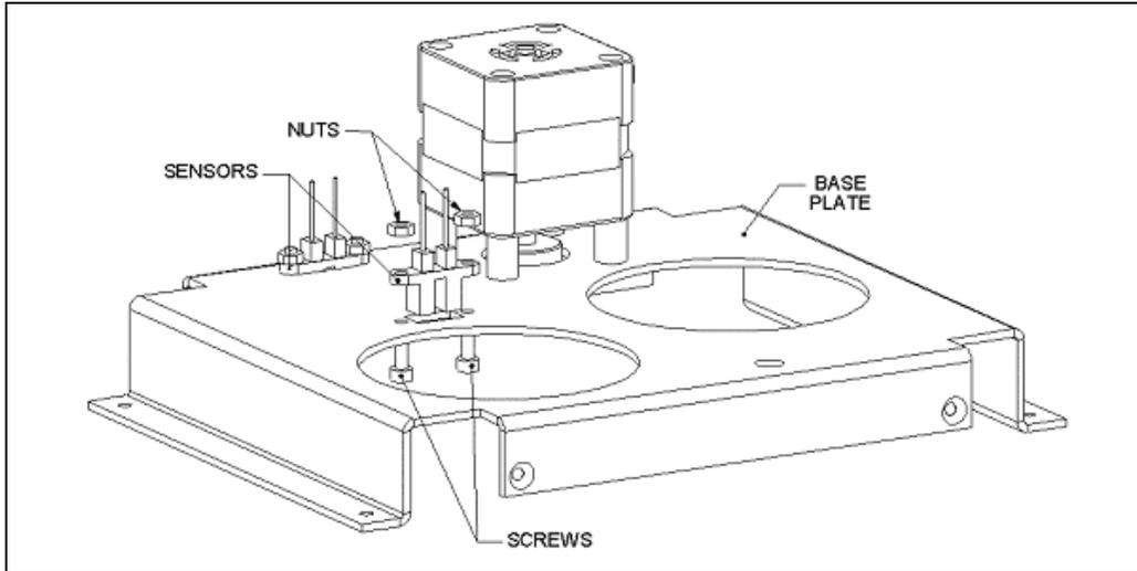
Figure 13-28 Mounting the Sensor Assemblies
