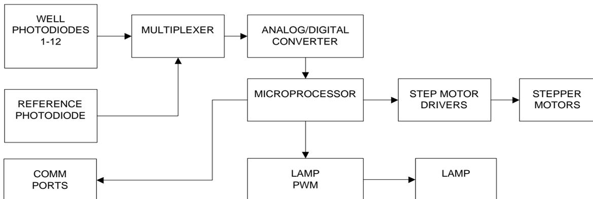
Figure 10-2 Functional Diagram of the Reader Module
