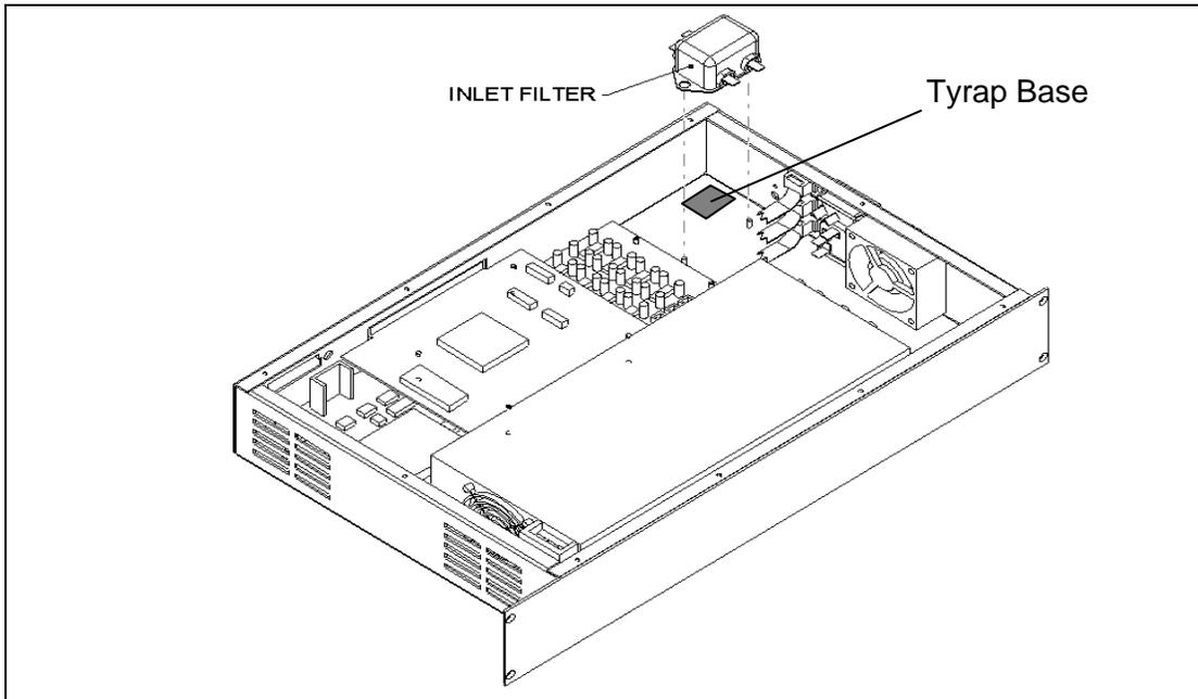
Figure 17-6 Inlet Filter
