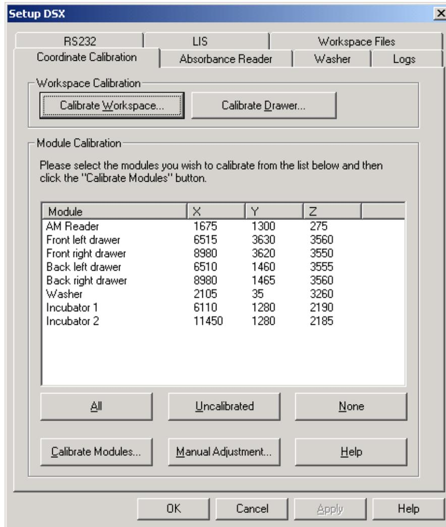
Figure 3-2 Setup DSX Dialog Box - Coordinate Calibration Tab
