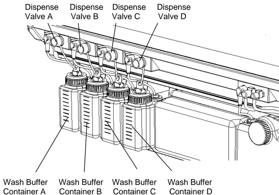
*Figure 1-9 Wash Buffer Containers and Wash Buffer Dispense Valves*
