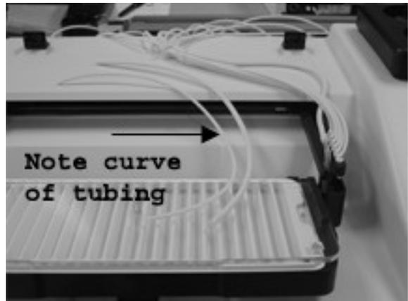
Attach the tubing for Pump 1 to the dispense tip as shown to the right.
