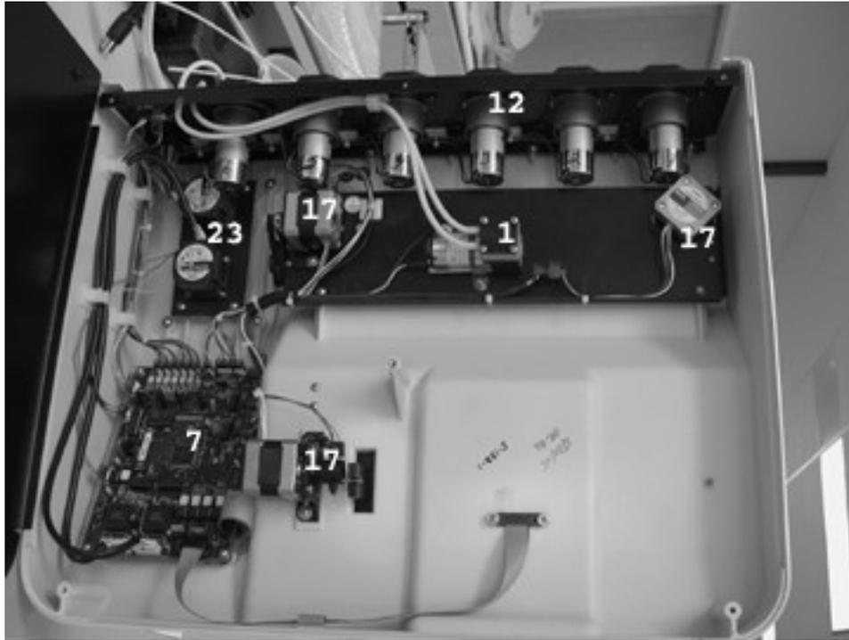
**Inside Enclosure: #1 Aspirate Pump, #7 Circuit Board, #12 Peristaltic Pump (Dispense), #17 Stepping Motor, #23 Stirrer Motor**
