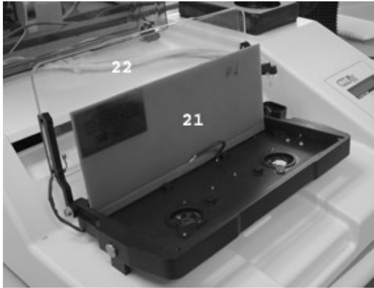
**#21 Platform Heater Assembly, #22 Condensate Shield Assembly**
