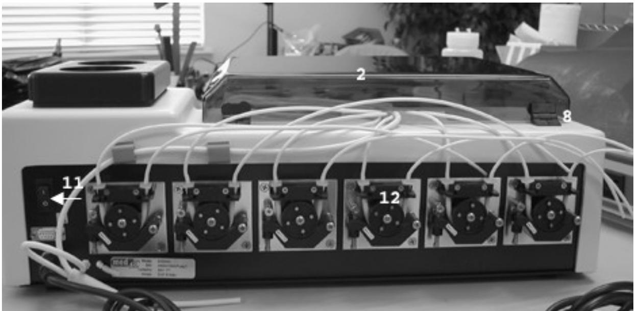
**#2 Aspirate Shield, #8 Hinge, #11 On/Off Switch, #12 Dispense Pump**
