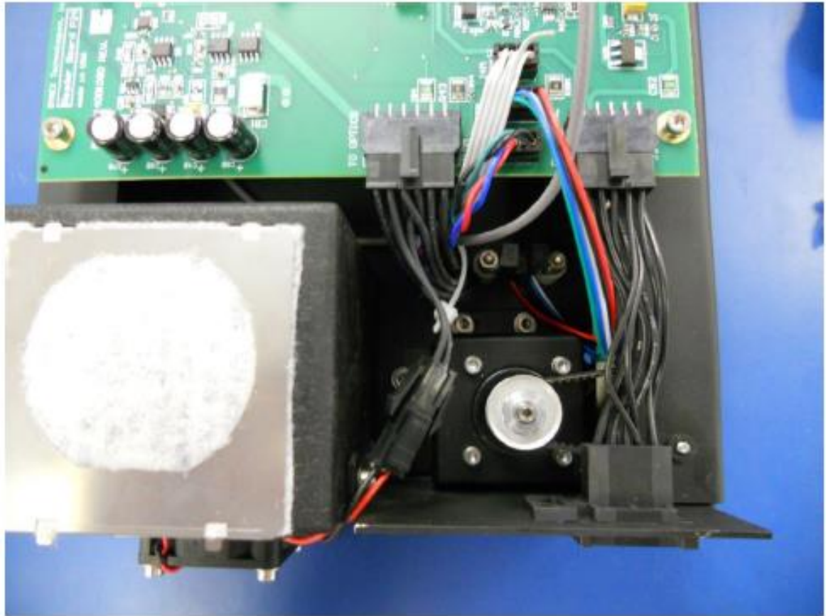
Figure N-8: Cables on the Reader PCB
