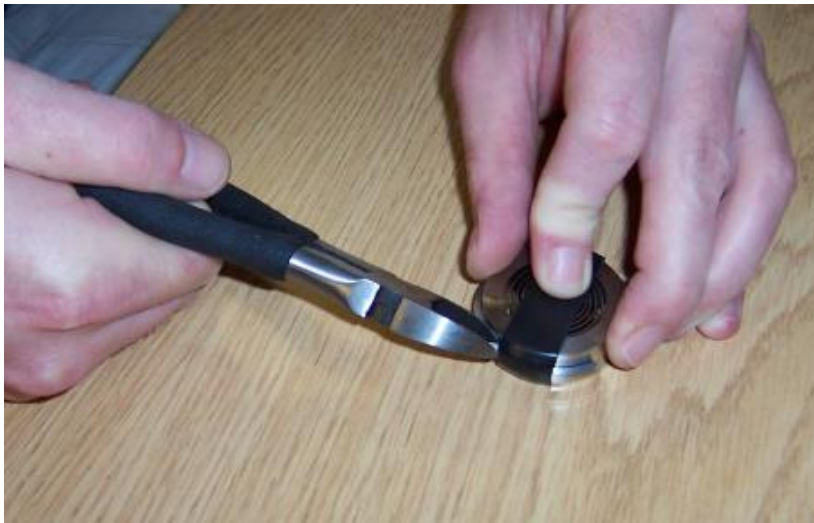
Figure Z-26: Removing Heat Shrink
